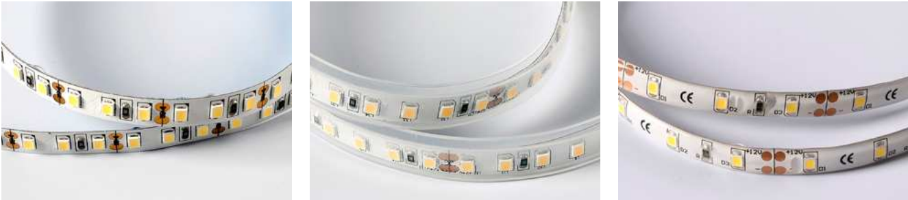
A. 裸灯带 IP20, 建议使用 功率范围 8-16W/M Type A. IP20. Bare LED light strip has power range 8 ~ 16 W/M. B. 套管灯带 IP65，建议使用 功率范围 8-12W/M Type B. IP65. Silicone tube encased LED light strip has power range 8 ~ 12 W/M. C. 滴胶灯带 IP54，建议使用 功率范围 8-12W/M Type C. IP54. Silicone coated led LED light strip has power range 8 ~ 12 W/M.
